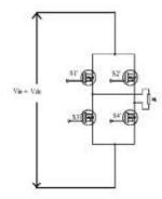
Fig.4.Circuit diagram of single phase full bridge inverter The switching scheme used for the inverter section is shown in the table given below.
