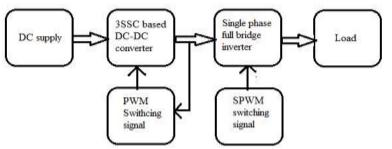
Fig.1.Block diagram of the proposed topolgy
