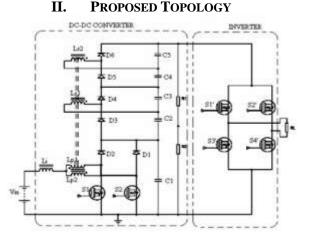
Fig.2. Circuit diagram of the proposed topolgy
